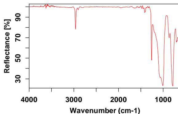
Figure 4. ATR Spectrum of Silicone Rubber Tape.
