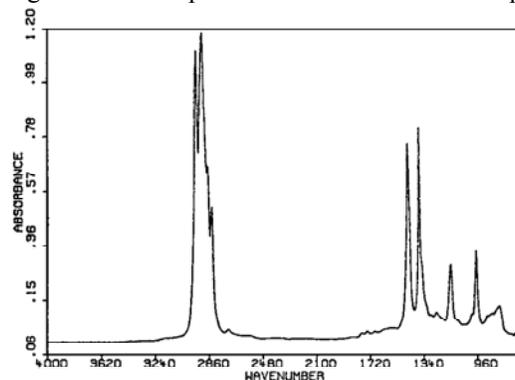
Figure 5. ATR Spectrum of Anhydrous Maleic Acid in Molten Polypropylene Recorded at 185°C.
