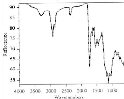
Figure 4. ATR Spectrum of an Adhesive on Paper.
