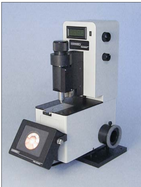
Figure 1. The VideoMeridian™ viewing diamond ATR with optional video display.
