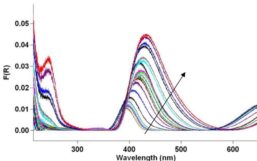
Figure 3. Diffuse Reflectance Spectrum of NiSO<sub>4</sub> at temperature from 20°C to 180°C, with the arrows showing increased temperature trends.
