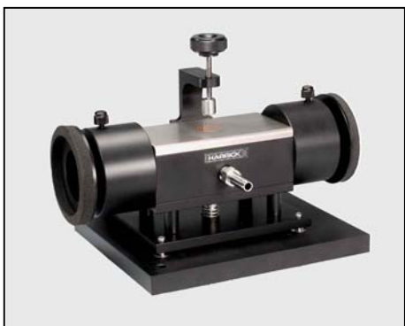
Figure 2. The FastIR™ Accessory: 45° ATR with ZnSe crystal.
