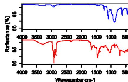
Figure 7. ATR spectrum of blue grip (red) and the thrust device (blue),
