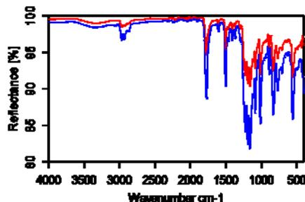
Figure 5. ATR Spectrum of the body (red) and the push button (blue).
