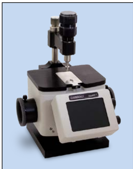
Figure 1. The VideoMVP™ Single Reflection Diamond ATR Accessory.
