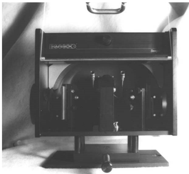
Figure 3. Seagull™ variable angle reflection accessory with ATR kit and liquid cell installed.
