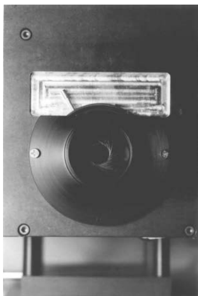
Figure 1. Diaphragm aperture installed in the entrance beam side of the Seagull TM .
