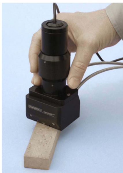
Figure 1. The Omni-Diff diffuse reflection fiber optic probe with its digital camera.
