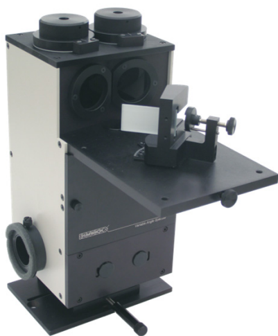
Figure 1. The Variable Angle Reflection Accessory with its Variable Angle Stage.
