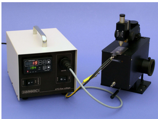
Figure 1. The Meridian SplitPea with its Heated Diamond Sampling Plate and Temperature Controller.
