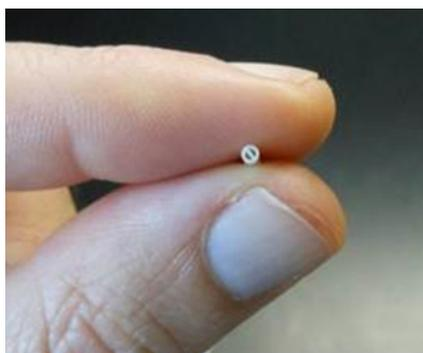
Figure 2. Cross-section of a 5 French dual lumen CVC showing the approximate size of the inside surfaces requiring consistent and precise ATR FT-IR.
