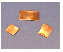
Figure 4. The three coated copper chips.
