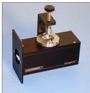
Figure 3. AccessATR single reflection ATR accessory.
