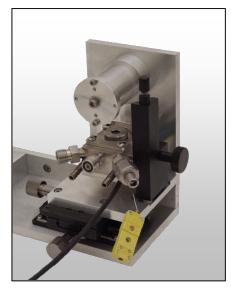
Figure 1. The Harrick Emission Accessory with the Harrick Heated Vacuum Chamber (HVC) being used as the sample holder.
