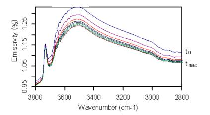
Figure 2. Spectra of kaolinite taken at 700  $^{\circ}\mathrm{C}$  in 10-minute intervals.
