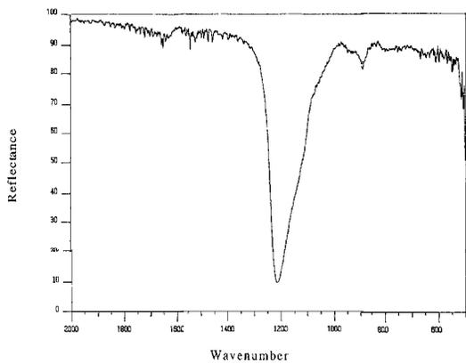
Figure 2. Spectrum of SiO<sub>2</sub> on an Al Substrate
