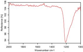
Figure 4. Specular reflectance of a 500 Å SiO coating on Al measured with a CIR fiber.
