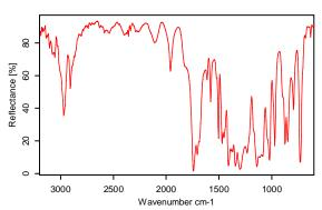
Figure 3. Specular reflectance of a 12  $\mu$ m mylar film on an Al mirror measured with a PIR fiber.
