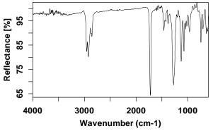
Figure 5. ATR Spectrum of a Plastic Toy Fish.
