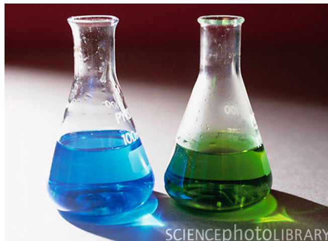
Figure 3. Copper sulfate solution before (left) and after (right) the addition of hydrochloric acid.
