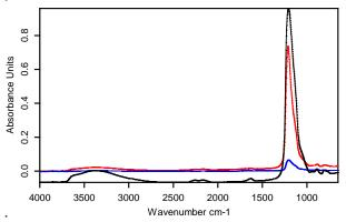
Figure 2. The spectra of a 100Å coating of MgF<sub>2</sub> on gold acquired via 45° single reflection (blue), 75° single reflection (red), and the BoostIR<sup>™</sup> (black).
