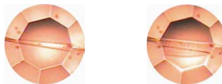
Figure 2. Photographs of the 20 \mu\text{m} PET Fiber compressed with 20 (left) and 302 (right) units of pressure.
