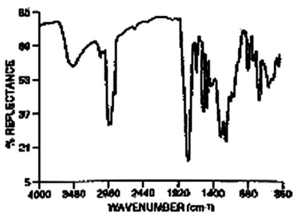
Figure 5. Internal Reflectance of a Paint Chip.
