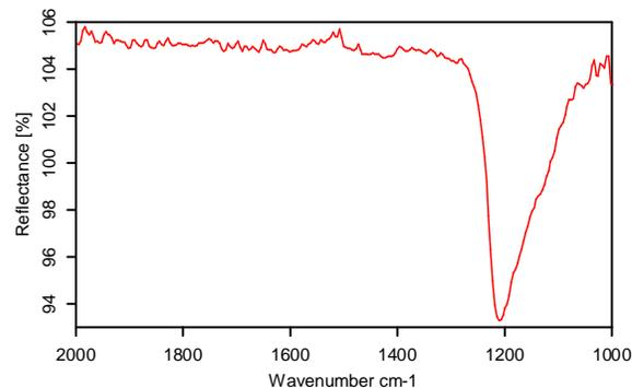
Figure 4. Specular reflectance of a 500  $\text{\AA}$  SiO coating on Al measured with a CIR fiber.
