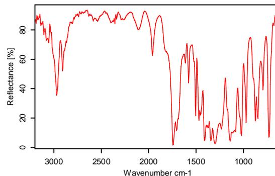
Figure 3. Specular reflectance of a 12  $\mu\text{m}$  mylar film on an Al mirror measured with a PIR fiber.
