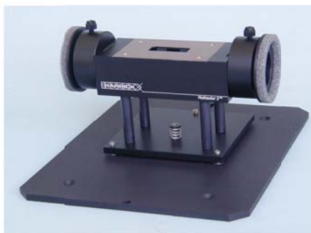
Figure 5. The Refractor2 is a fixed 75° accessory with a built-in polarizer used to examine thin films on reflective substrates.
