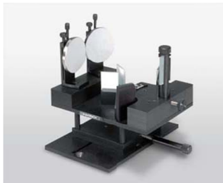
Figure 4. This variable angle specular reflection accessory, with the addition of a polarizer, is particularly useful for grazing incidence experiments to study thin films on metal surfaces.
