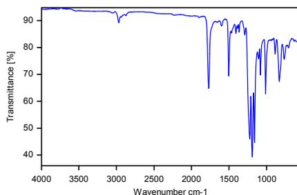
Figure 2. ATR Spectrum of the Cleaned Plastic Substrate.
