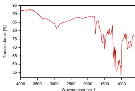
Figure 3. ATR Spectrum of the Coated Plastic.
