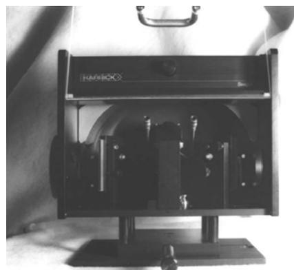
Figure 3. Seagull<sup>TM</sup> variable angle reflection accessory with ATR kit and liquid cell installed.
