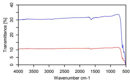
Figure 10. Seagull™ throughput without accessory aperture (top) and with accessory aperture (bottom).
