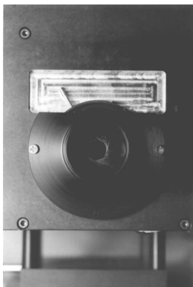
Figure 1. Diaphragm aperture installed in the entrance beam side of the Seagull™.
