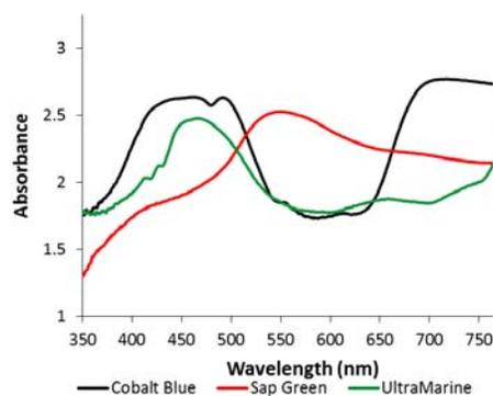
Figure 7. Diffuse Reflectance Spectra of the Blueish Samples.
