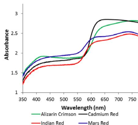
Figure 5. Diffuse Reflectance Spectra of the Reddish Samples.
