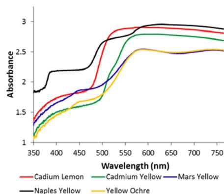
Figure 6. Diffuse Reflectance Spectra of the Yellowish Samples.
