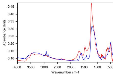
Figure 2. Grazing angle reflectance spectra of two coated steel rivets.
